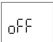
After logger expired, logger enters power off status and show "off" on LCD when user attempts to program or start the expired and unused logger.
